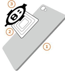
(a) The sticker for the visitors' OD (1) includes an RFID tag (2) as well as a visual marker (3). The visual marker and the RFID tag is needed to identify the visitors' OD at the various active exhibits. If the exhibit is, e.g., a capacitive table, the visitors' OD can register itself by means of RFID readers installed at the table. If the exhibit uses an optical approach (e.g., optical table), the visitors' OD can be identified by its visual marker.
