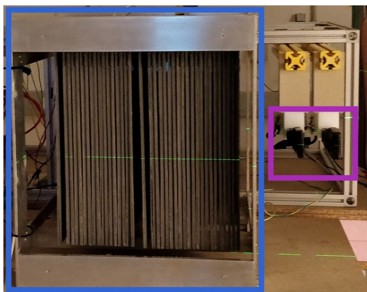
Figure 20: Photo of the measurement set-up, trigger marked with a violet rectangle and calorimeter marked with a blue rectangle. The beam's projected trajectory is indicated by the green laser.
