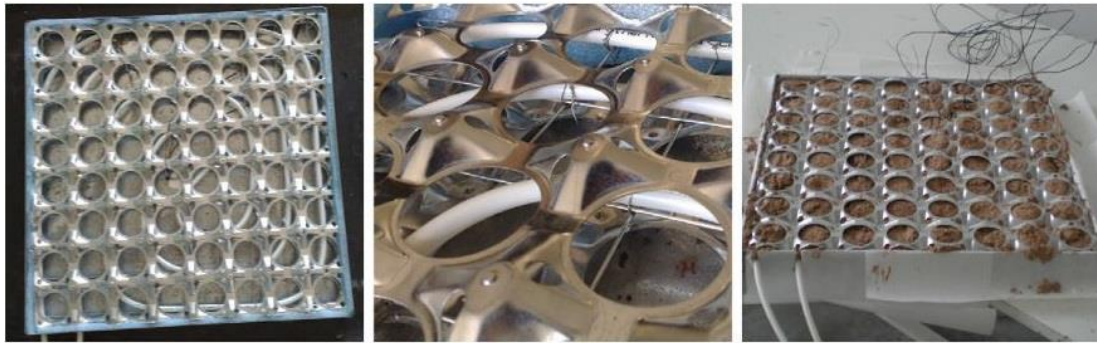
Figure 4-9: steel matrix for increased structural strength and conductivity (Ansuini et al. 2011)
