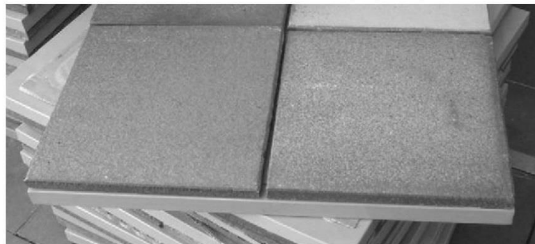
Figure 4-11: PCM-tile prototype (Cerón et al. 2011)
