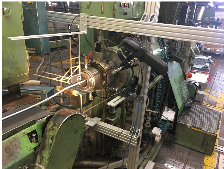
Fig. 1.2: Picture of a screw extruder used at Semperit Technische Produkte GmbH, additionally equipped with the measuring equipment used in the experimental campaign described in Chapter 2 of this thesis
