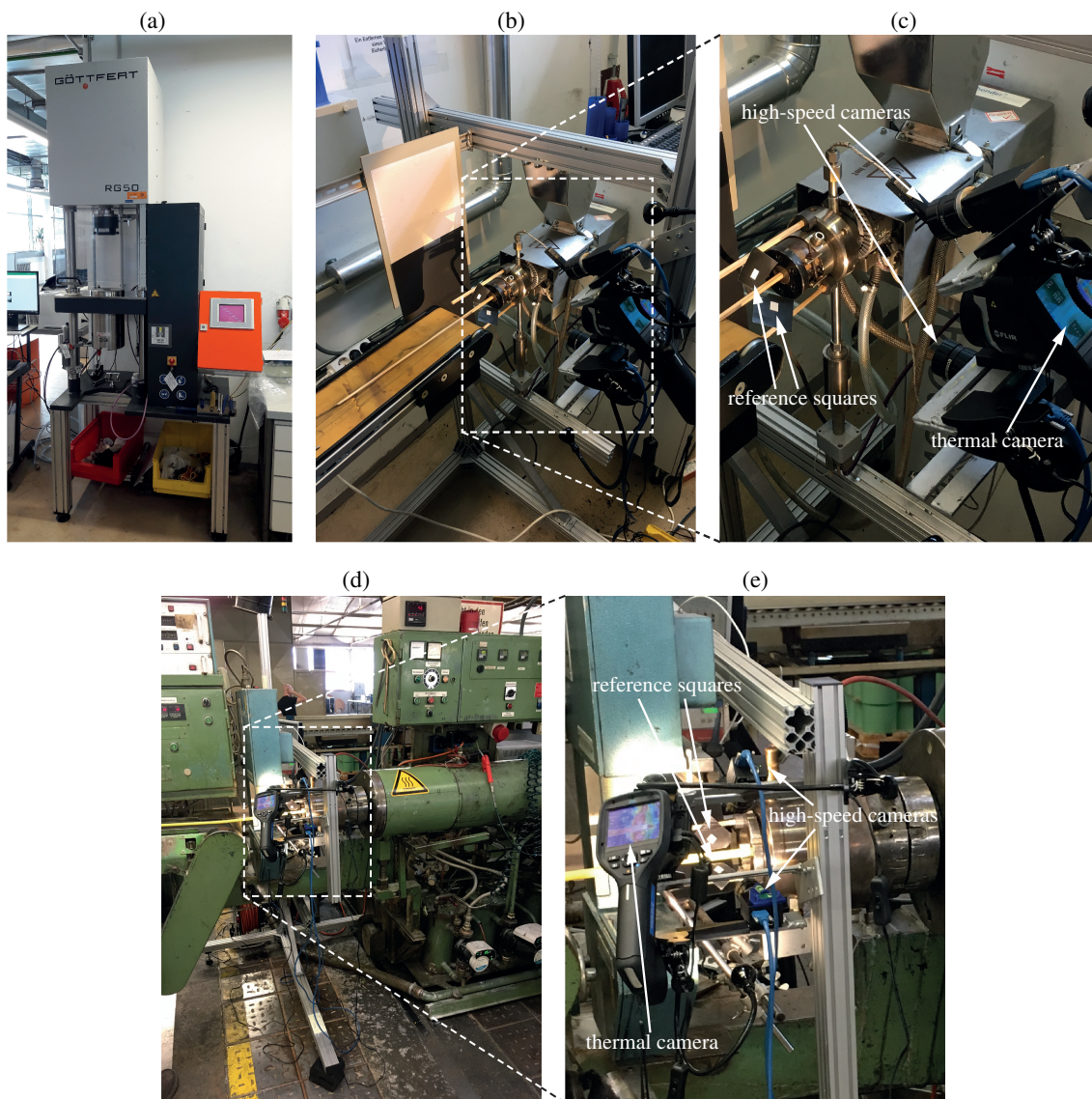
Fig. 2.4: Extrusion facilities used in this study, comprising (a) a Göttert Rheograph 50, (b) a laboratory extruder of type Brabender Plastograph, (c) a magnified area of (b), (d) a production extruder, and (e) a magnified area of (d). The mounted measuring equipment (i.e., high-speed cameras, thermal cameras, and reference squares for subsequent evaluation) is indicated in (c) and (e).
