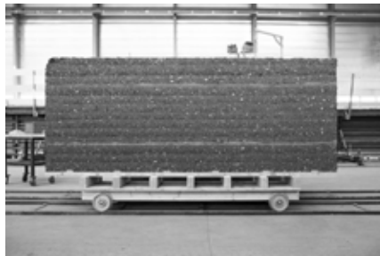
Finished prefabricated wall element ill.[75]
