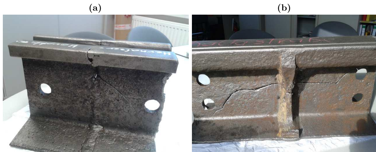
Fig. 1.1: Typical crack patterns occurring in grooved rails of the Viennese tramway network; (a) transverse crack in the rail head; and (b) crack pervading the rail in longitudinal direction; by courtesy of WIENER LINIEN
