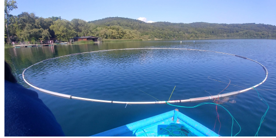
Figure 3.4: Assembled TEM-loop during field work at Laacher See, Germany.
