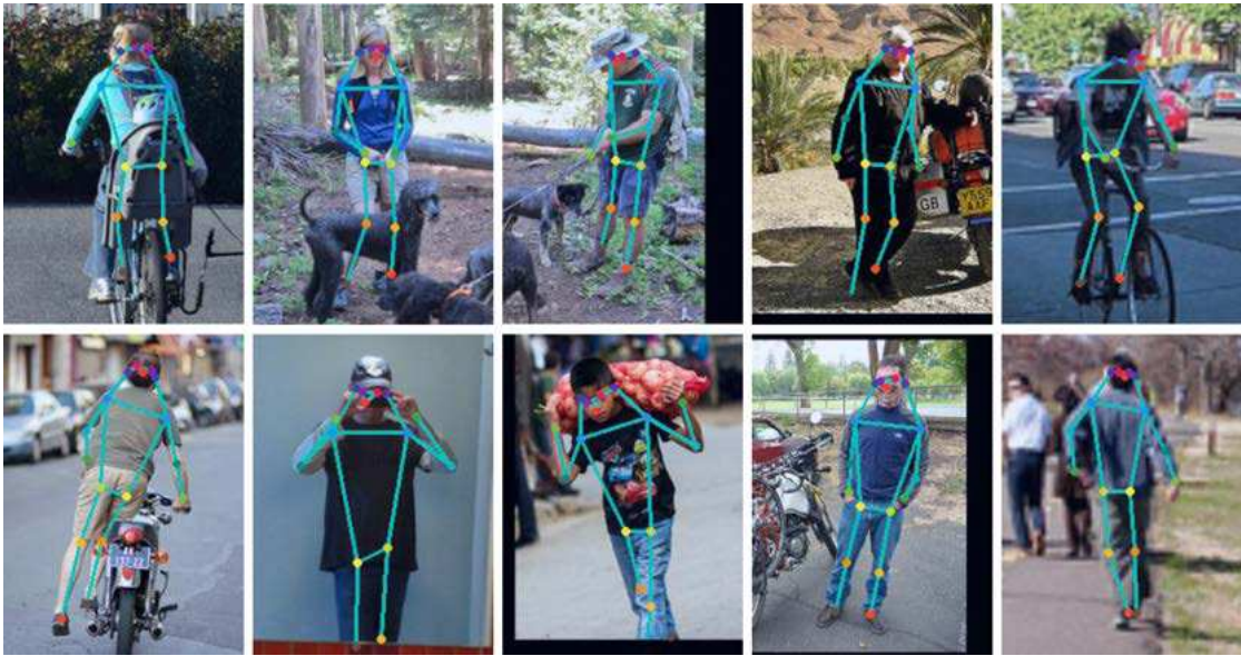
Figure 4.1: A selection of COCO images with accurate predictions by the algorithm which was trained on the main dataset. Colored dots represent predicted joint positions. A specific color relates to the type of predicted joint (e.g. red for the left ankle joint). Blue lines connect predicted joint positions to form a skeleton structure (e.g. the left wrist is connected to the left elbow). The predicted 2D joint positions for this selection of images worked particularly well and properly formed skeleton structures can be seen.
