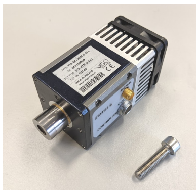
Figure 3.8.: Mercury-cadmium-telluride-based IR detector with an integrated Peltier-cooler and preamplifier (M6x25-screw for scale).
