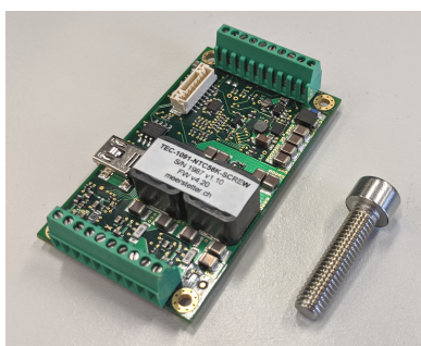
Figure 3.10.: Temperature controller TEC-1091 with an M6x25-screw for scale.
