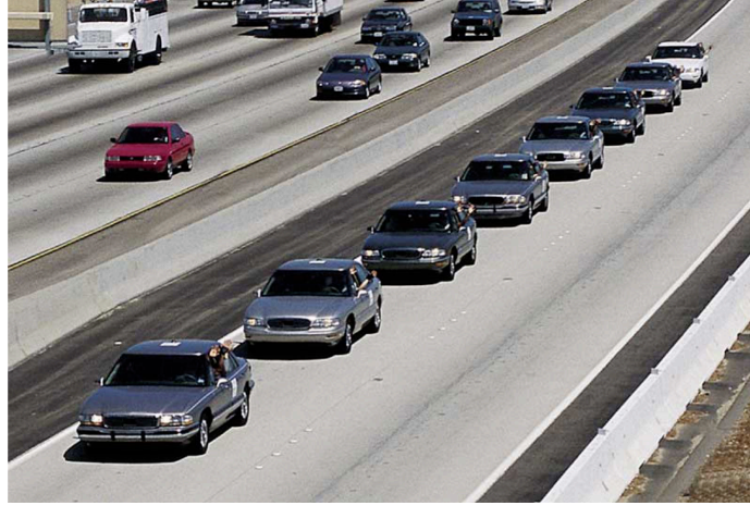
Figure 1.5: Eight-car platoon demonstration of the National Automated Highway Systems Consortium in San Diego, California, in 1997 taken from [31].
