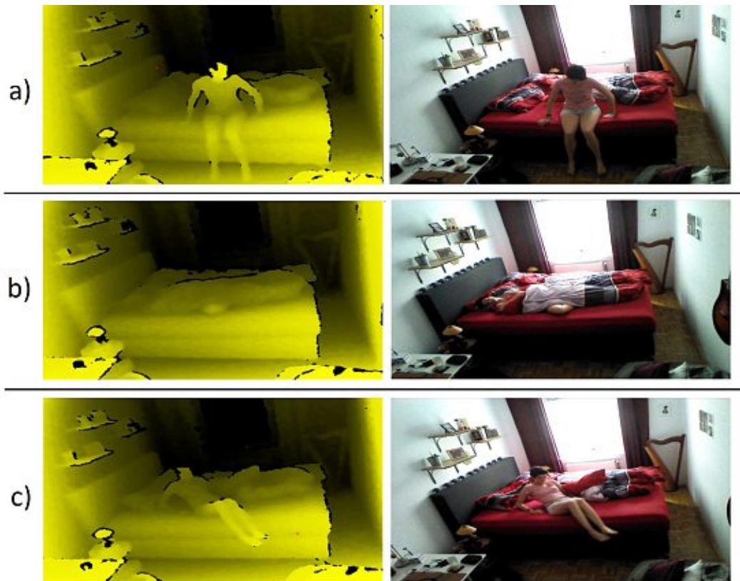
Figure 3.5: Example of an image which is a) labeled "standing" where a person is sitting on the edge of the bed and b) labeled "lying" where a person is lying on a bed; c) shows the critical point at which the position changes from lying to standing.
