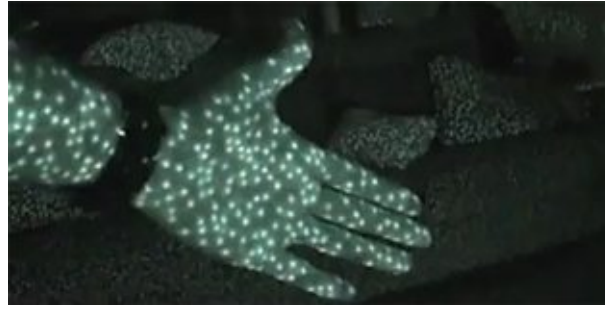
Figure 3.2: Illustration of projected dot pattern from an IR-projector into its field of view [103].
