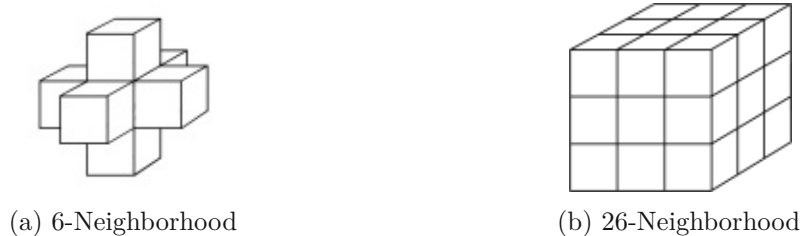
Figure 3.7: A scheme for the 6- and the 26-neighborhood of a voxel/element of a 3D matrix.
