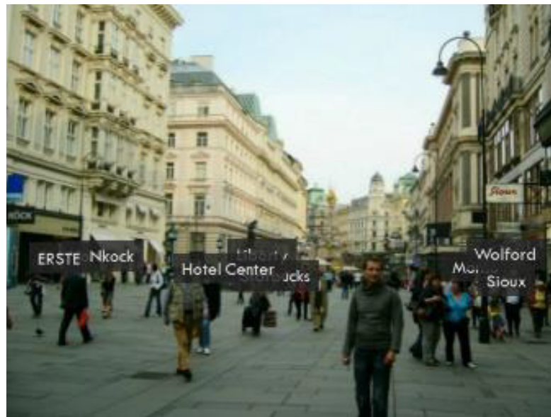
Figure 2.12: A street with labeled buildings by Jia et al. [JZWG18, p. 1658]. Labels of distant POIs may become occluded by close ones. The information (text in this case) cannot be retrieved from the occluded labels.
