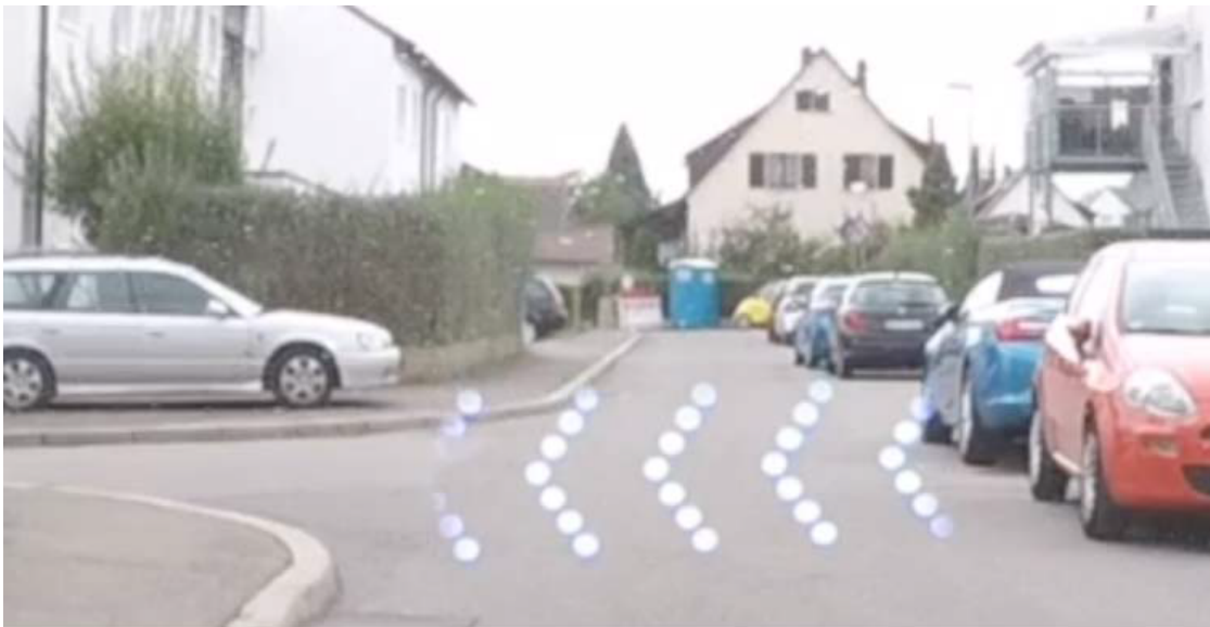
Figure 2.5: Explanatory result by Schneider et al. [SBN + 19, p. 360]. The white arrows help the drivers to navigate towards the destination. The arrows are projected onto the windshield of a car.
