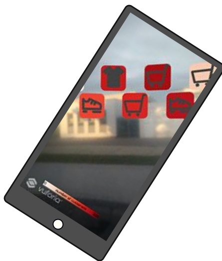
Figure 5.14: Tilted device showing the Local Shops Dataset . The labels stay perpendicular to the ground.
