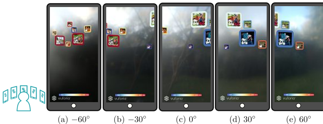
Figure 5.13: Labeling of the Tokyo Disneyland Dataset in AR. The images present results of different viewing angles to show consistent label positions when the AR device is rotated toward different directions by the user.
