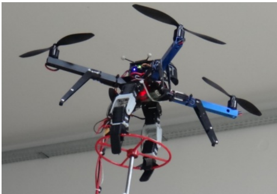
Figure 2.7: Aerial vehicle with 2-DOF manipulators turning a valve [KOO14].
