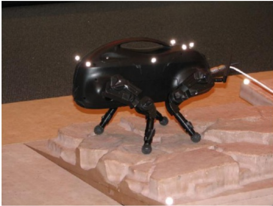
Figure 2.5: LittleDog with markers on terrain board [CVGL07].
