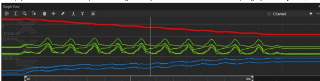
(b) x- (red), y- (green) and z-positions (blue) of the four FLbtm markers shown in Motive's Graph View.
