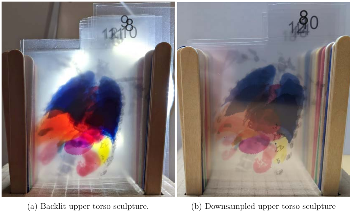
Figure 5.9: Two methods to improve the visibility of Vologram sculptures. The original sculpture is shown in Figure 5.8b (a) Viewing the sculpture in front of a light source improves the visibility of structures in slides further to the back of the figure. (b) Removing every second slide reduces the image resolution along the viewing axis, but structures in the back part of the volume can be seen better.
