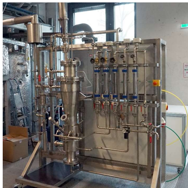
Figure 5: Picture of the bench-scale methanation setup at TU Wien
