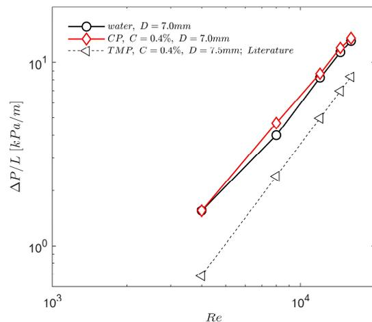
Figure 2: Pressure drop within the experimental setup (entrance channel  $D = 7\text{ mm}$ , 400 mm long + fractionator geometry) of the chemical pulp ( $D/L_1 = 3.15$ ),  $C = 0.4\%$  and pure water compared to the pressure drop of a TMP pulp in a  $D = 7.5\text{ mm}$  pipe ( $D/L_1 = 3.18$ ) [13].
