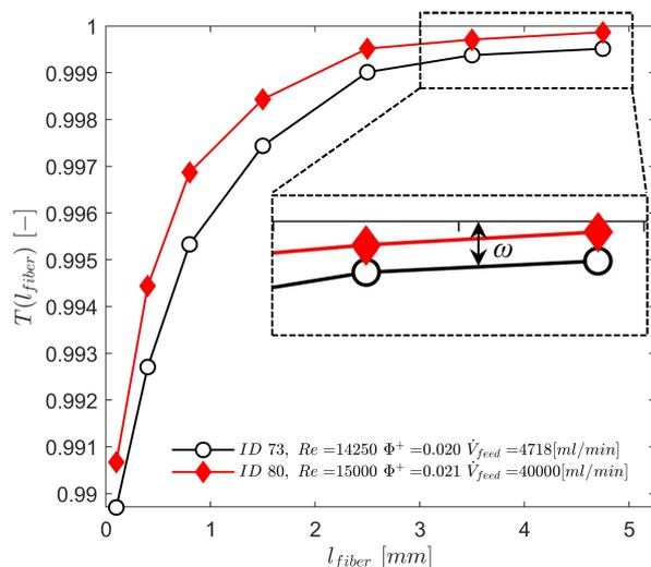
Figure 7: Grade efficiency curve of (i) a single-channel single-step experiment (ID73) and (ii) of an eight-channel single-step experiment (ID80) at both a channel Reynolds number of approx.  $Re = 15,000$ , a volumetric accept ratio of  $\Phi^+ = 0.02$  and an inlet consistency of both  $C = 0.5\%$ .
