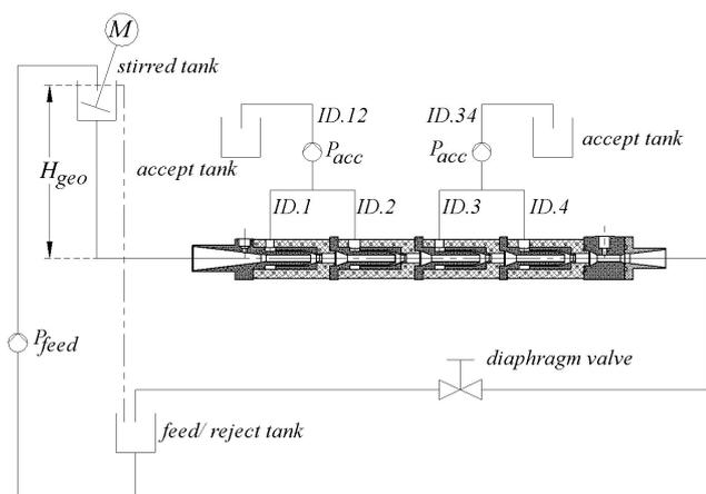
Figure 3: process diagram of the single-channel and four-step experimental setup including (i) a view of the fractionator itself, (ii) the pulp tanks for accept, feed/reject and for adjusting geodetic height upstream the fractionator, and (iii) the accept and feed pumps, both peristaltic pumps to exactly adjust flow rates.
