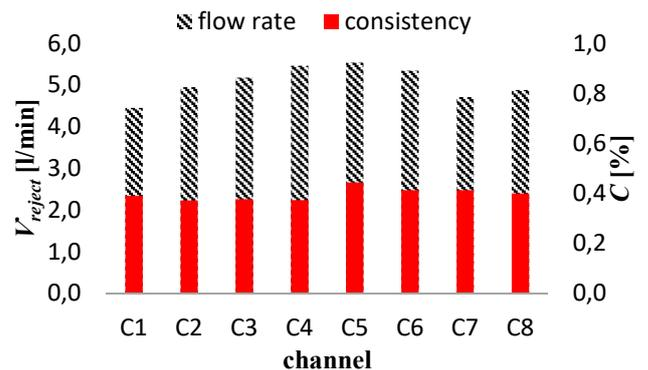
Figure 6: Reject flow rate measurement and consistency distribution over all eight fractionation channels of the eight-channel fractionator.
