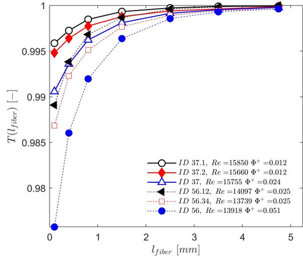
Figure 5: grade efficiency curve of (i) a single-channel two-step experiment (ID37) including the grade efficiency curves for each step (ID37.1 and ID37.2) with a feed consistency of  $C = 0.6\%$  and (ii) grade efficiency curve of a single-channel four-step experiment (ID56) including the grade efficiency curves of steps one and two (ID56.12) and of steps three and four (ID56.34) with a feed consistency of  $C = 0.5\%$ .
