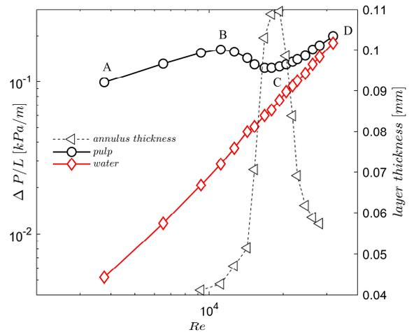
Figure 1: Pressure drop of pure water (red diamonds) and a birch fiber suspension (black circles) flow in a pipe in plug flow regime,  $D = 0.04m$ , consistency  $C = 1.0\%$ , including measured annulus thicknesses, data published by Jäsberg [16].
