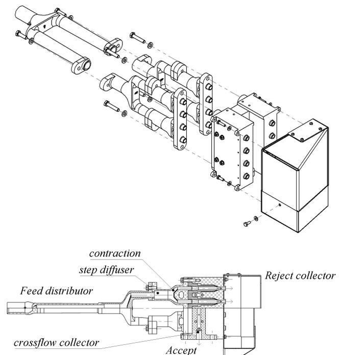
Figure 4: prototype of a multi-channel fractionator including (i) a feed pulp distributor, (ii) the fractionation section including an accept collector and (iii) a reject collector (free jet into a sheet metal box).
