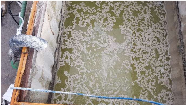
Fig. 3: Water jet cutting wastewater container
