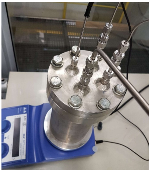
Figure 1. Heat treatment reactor.
