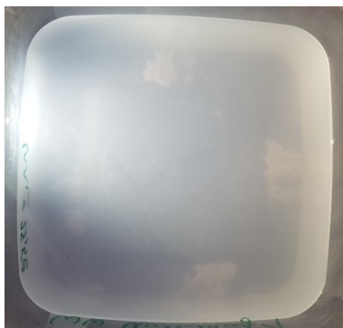
Fig. 8: Illuminated sample from the underflow with clearly visible fiber content
