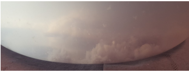
Fig. 2: "washing water" – sample with sedimented fibres
