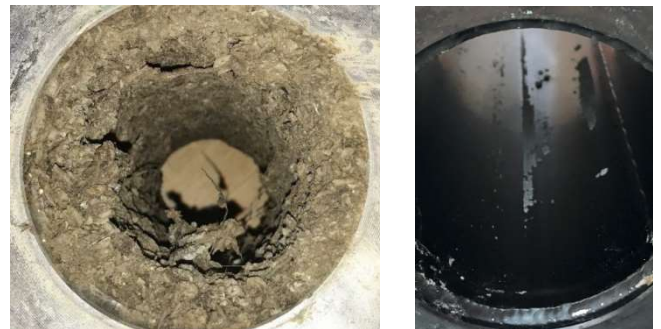
Fig. 8, Contaminations after campaign 03 and 04 (DLC)
