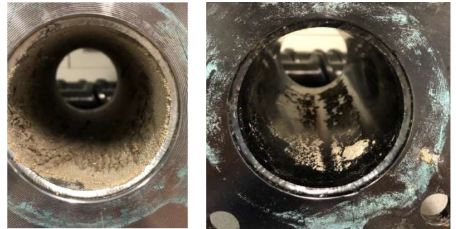
Fig. 6, Contaminations after campaign 01 and 02 (DLC)
