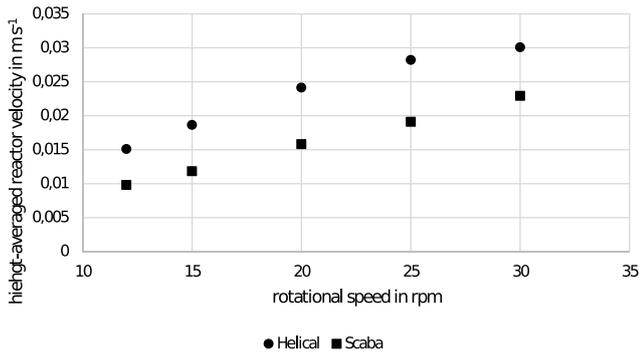
Figure 6: Comparison of the height-averaged velocities inside the reactor for both helical and Scaba at different rotational speeds. Experimental setup shown in Figure 5. ( $w_{\text{glyc}} = 75 \text{ wt\%}$ ,  $T = 21 \text{ }^\circ\text{C}$ ,  $\eta = 0.0343 \text{ Ns m}^{-2}$ ,  $\rho = 1193.7 \text{ kg m}^{-3}$ )
