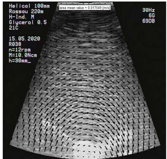
Figure 2: Illustration of captured and evaluated ultrasonic flow field in X-Y-plane. 50 wt% glycerol-water mixture with a helical stirring device (100 mm) at 12 rpm is used.
