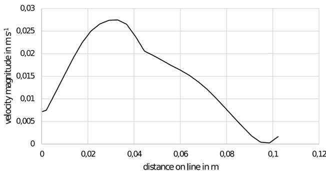
Figure 7: Illustration of the velocity profile along a centric polyline in reference to Figure 2 at a reactor height of 0.3 m. Velocity profile starts at stirring shaft (Distance on line = 0 m) and ends at the reactor wall (Distance on line = 0.11 m).
