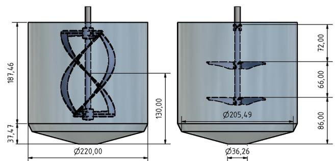
Figure 1: Laboratory scaled reactor with 1) helical and 2) Scaba agitation device (dimensions in mm)
