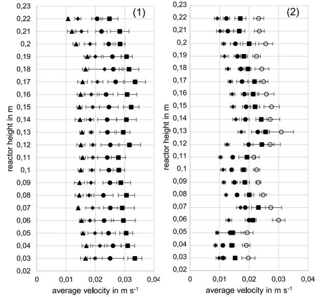
Figure 4: Flow field evaluation in a two-component glycerol/water-mixture with different agitation speeds using (1) a helical stirring device (100mm) and (2) a Scaba device. ( $w_{glyc} = 50\text{ wt}\%$ ,  $T = 21\text{ }^{\circ}\text{C}$ ,  $\eta = 0.0058\text{ Ns m}^{-2}$ ,  $\rho = 1126.3\text{ kg m}^{-3}$ ) ▲: 12rpm, ◆: 15rpm, ●: 20rpm; ■: 25rpm; ○: 30rpm
