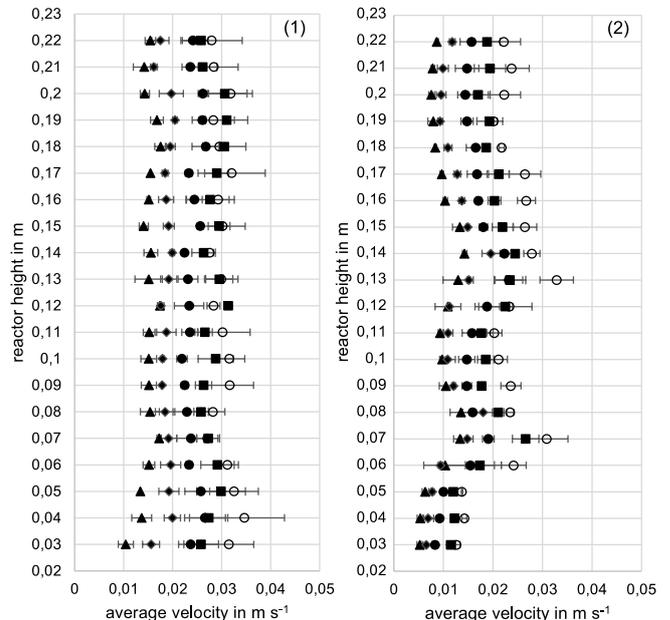
Figure 5: Flow field evaluation in a two-component glycerol/water-mixture with different agitation speeds using (1) a helical stirring device (100mm) and (2) a Scaba device. ( $w_{glyc} = 75\text{ wt}\%$ ,  $T = 21\text{ }^{\circ}\text{C}$ ,  $\eta = 0.0343\text{ Ns m}^{-2}$ ,  $\rho = 1193.7\text{ kg m}^{-3}$ ) ▲: 12rpm, ◆: 15rpm, ●: 20rpm; ■: 25rpm; ○: 30rpm
