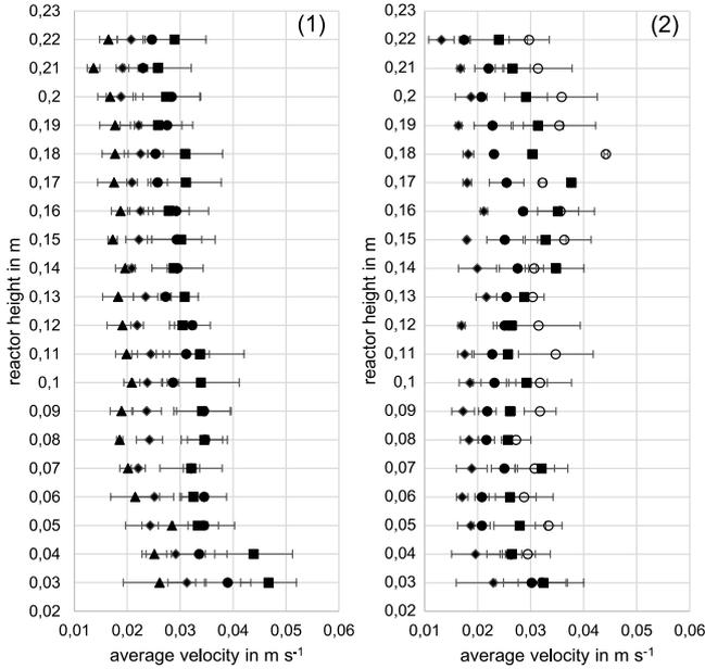
Figure 3: Flow field evaluation in pure water with different agitation speeds using (1) a helical stirring device (100mm) and (2) a Scaba device. ( $w_{glyc} = 0wt\%$ ,  $T = 21\text{ }^{\circ}\text{C}$ ,  $\eta = 0.00098\text{ Ns m}^{-2}$ ,  $\rho = 997.83\text{ kg m}^{-3}$ ) ▲: 12rpm, ◆: 15rpm, ●: 20rpm; ■: 25rpm; ○: 30rpm
