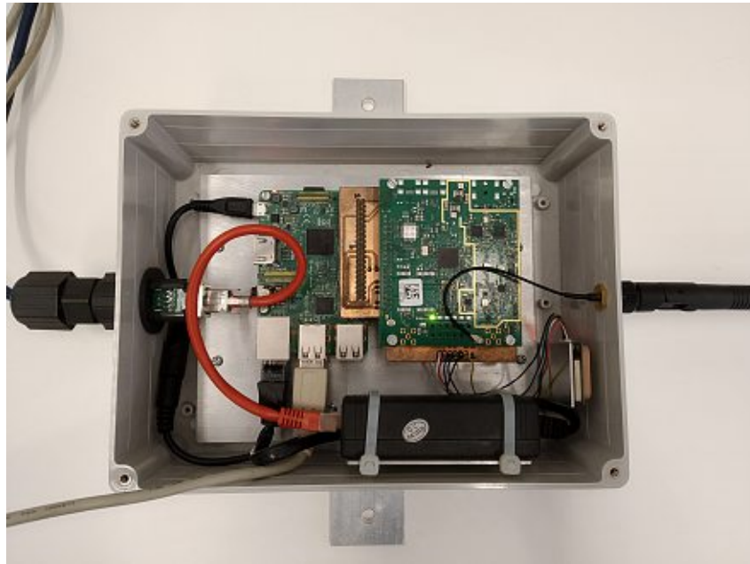
Figure 3.1: Gateway: Raspberry Pi 3 with IMST iC880A-SPI-LoRaWAN concentrator
