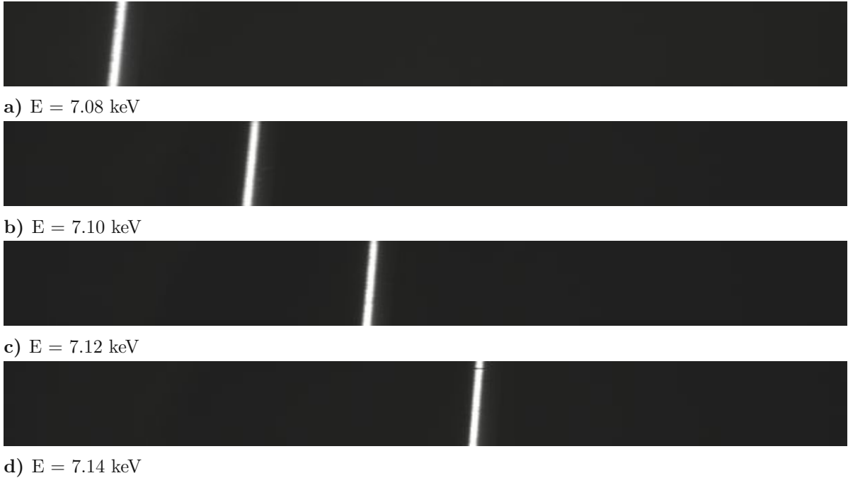
Figure 3.21: Monochromatic beams result in single lines on the CCD screen. For the energy calibration, several different energies are recorded.
