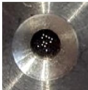
Figure 4.15: Mask in its holder. The 12 holes are drilled in a 25 mm thick platinum foil. The foil is placed into a holder manufactured for this purpose that can be screwed into the optics mounting of the camera.
