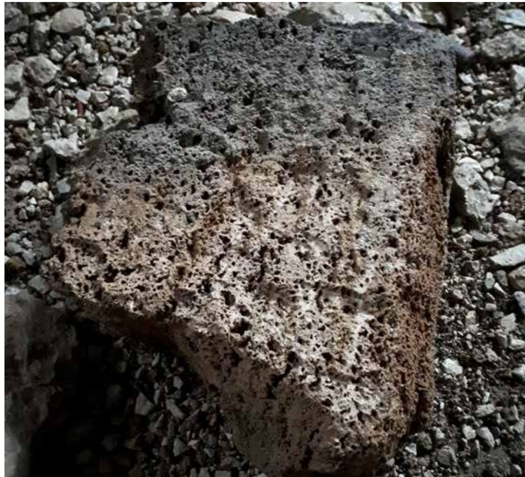
Fig. 65: The rock type used for the vaults inside (local "Siga") Credits: Ivan Vratnica
