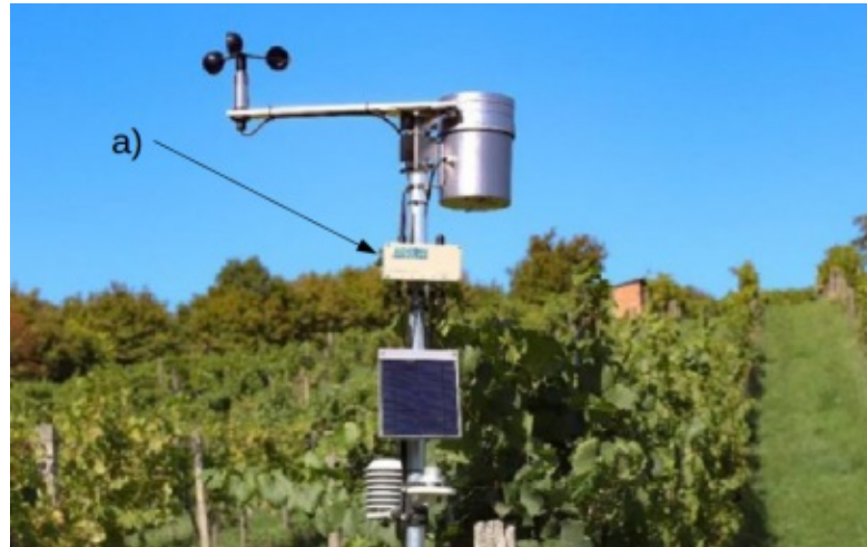
Figure 2.14: Adcon Weather Station [Apcb]. a) is the main part called ADCON RTU.
