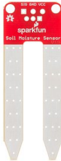
Figure 2.8: Resistor-based soil moisture sensor board from Sparkfun [Elea].
