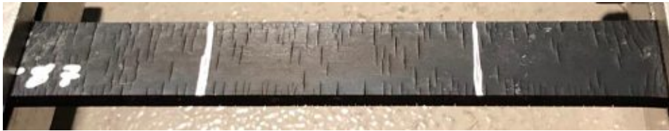
Figure 4: cracks perpendicular to the direction of strain on an ozone exposed rubber specimen
