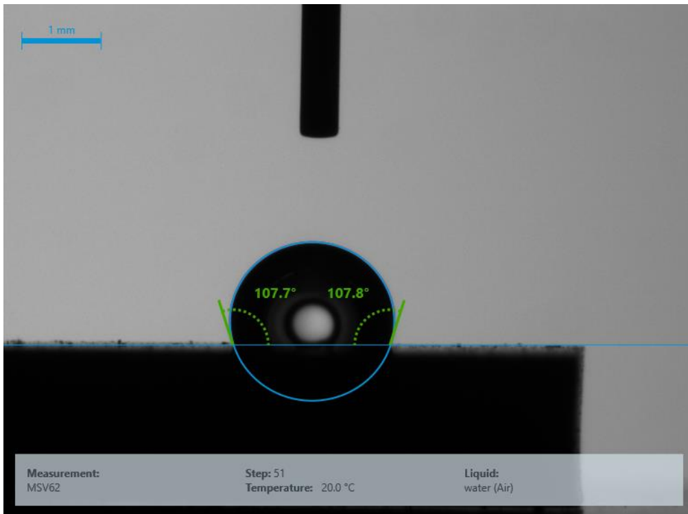
Figure 16: contact angle measurement between for 2 hours pre-passivated (200 pphm, 30 °C, 55 % RH) rubber and water
