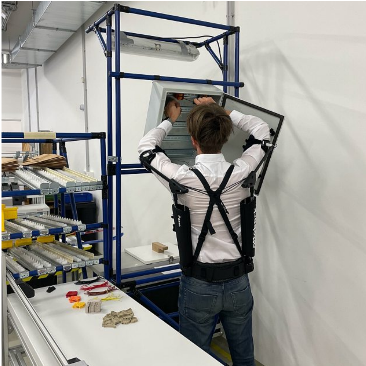
Abbildung 29: Ottobock Paexo Shoulder, Montage Use-Case
