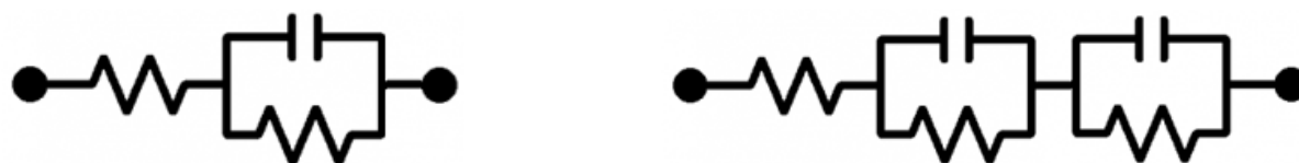
Figure 4-16: Equivalent circuit modelling to the obtained data. CHEX-10, CHEX-23, CHEP-10, CHEP-23, PG-10 and PG-23 data can be described with the left equivalent circuit, while CHEX-30 and PG-30 are described with the right equivalent circuit model [66, 68].
