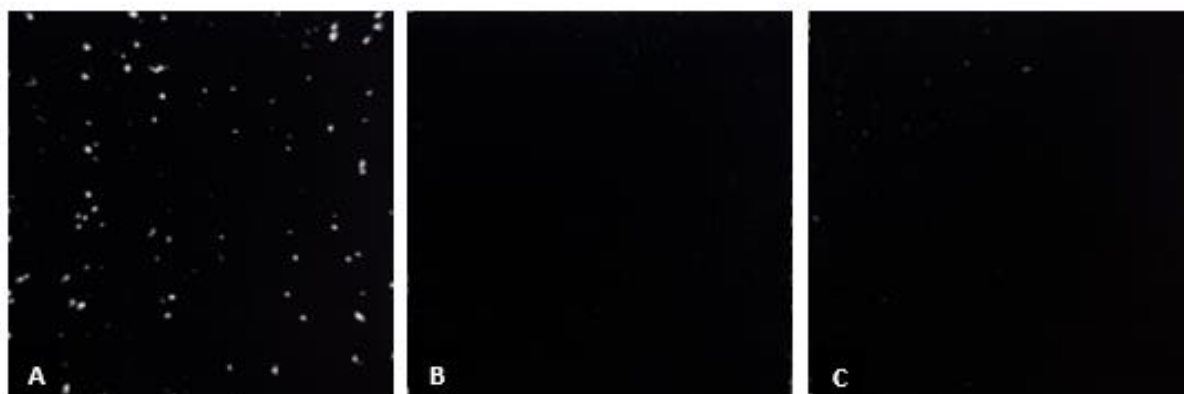
Figure 4-3: Comparison of the CCMs with 10 wt% ionomer in the dried CL. A: 50:50 CHEX:PG, B: PG, C: 50:50 CHEP:PG
