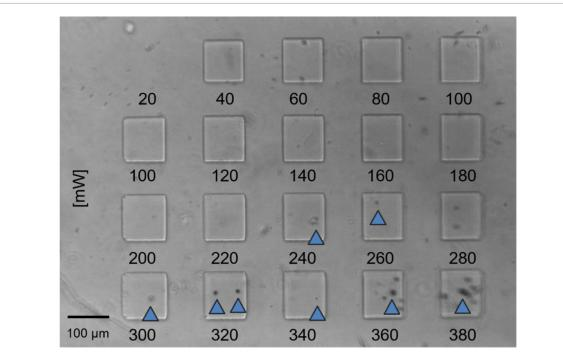
**Figure 2.** Optimization of two-photon polymerization (2PP) threshold for the PTMC-MA based resin. Microscopic visualization of cubes ( $100 \times 100 \ \mu$ m) printed using 2PP with increasing power intensities from 20 to 380 mW. The occurrence of bubbles inside the PTMC-MA due to thermal effects is denoted with the blue triangles.
