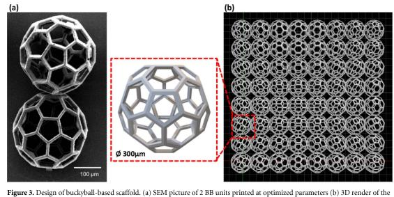
**Figure 3.** Design of buckyball-based scatfold. (a) SEM picture of 2 BB units printed at optimized parameters (b) 3D render of the scatfold consisting of an 8 × 8 × 3 array (l, w, h) of BB units with a diameter of 300  $\mu$ m each. The final size is 2.4 × 2.4 × 0.9 mm (l, w, h).
