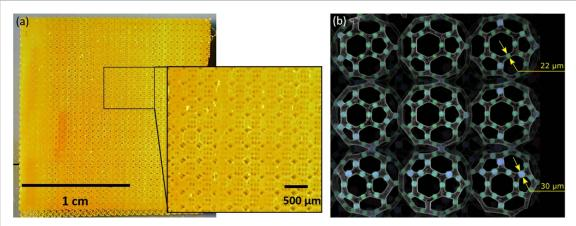
**Figure 5.** Upscaled scaffold printed using 2PP (a) Macroscopic observation of the large 2PP printed scaffold with a side length of 18 mm (b) Micro-computed tomography with overlaid spheres visualizing the local strut thickness.
