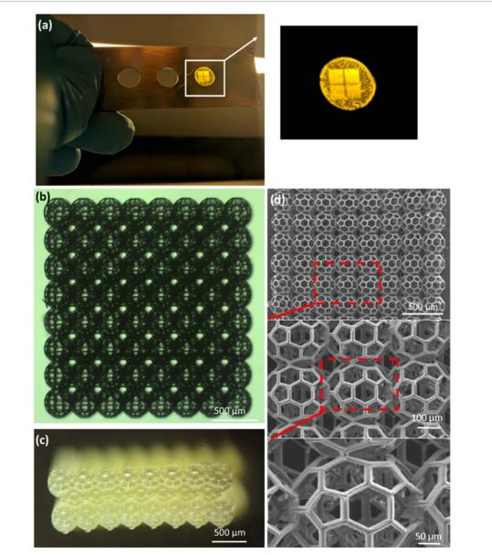
**Figure 4.** Scaffolds produced with 2PP (a) Illustration of the sample holder used for 2PP structuring containing 4 scaffolds still embedded in the unpolymerized resin. Macroscopic (b) top view and (c) side view of the tri-layered PTMC-based scaffold. (d) SEM images of the scaffold at various magnifications (x50, x150 and x300).
