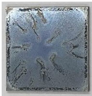
Figure 3-4: An actual photo showed the bad coatability of Ti_7O_4(OEt)_{20} spin-coated on a silicon wafer.
