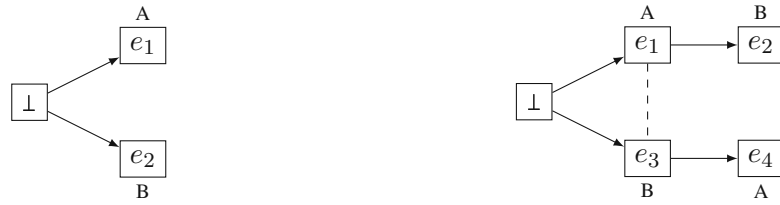
(a) An event structure with one maximal configuration. (b) An event structure with conflicts.
