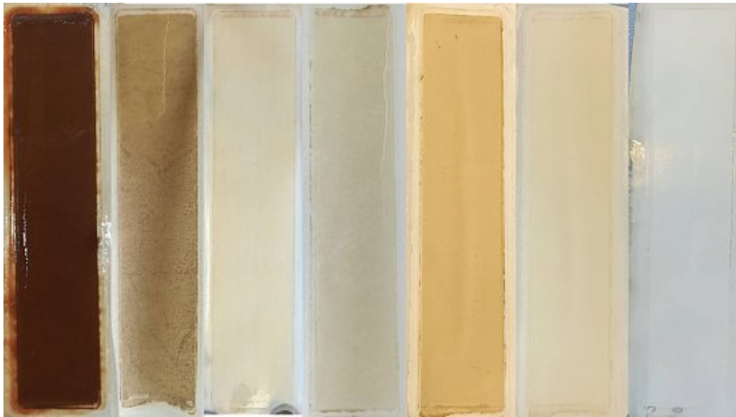
Figure 3.34: Membranes after use from left to right, M183, M180, K328, P707, UH050, UH020, RC10PE
