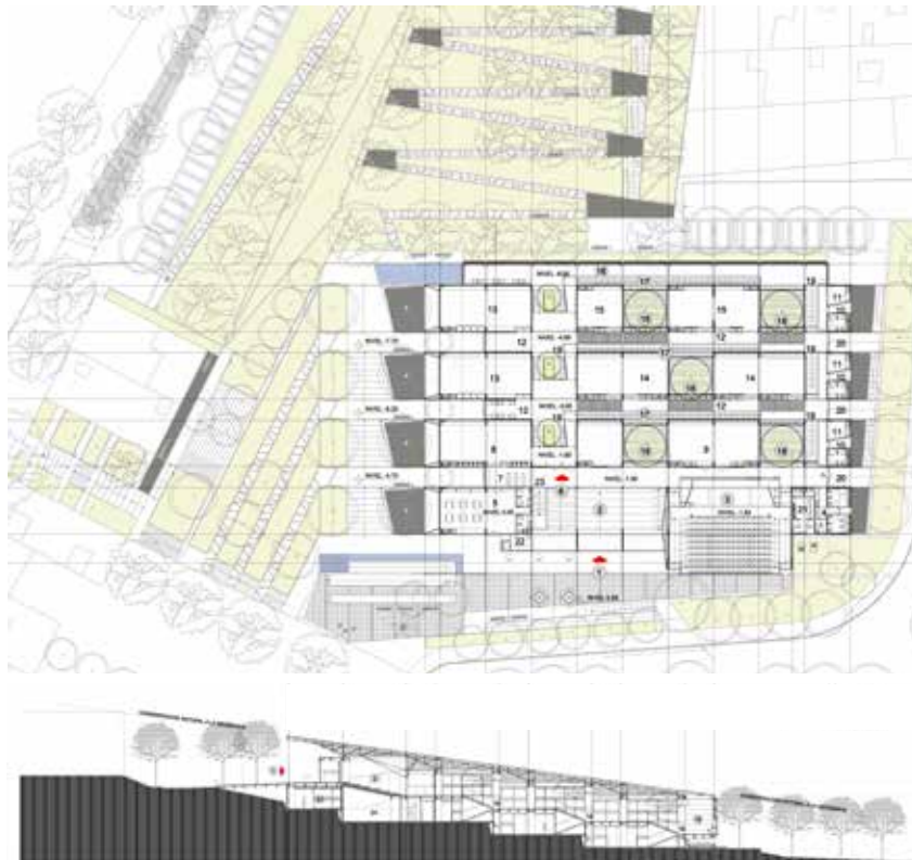
Fig 64-65. Ground Floor Plan and Section from the Parque Bibliotheca San Javier. [Graphics by JAVIER VERA ARQUITECTOS, 2006]
