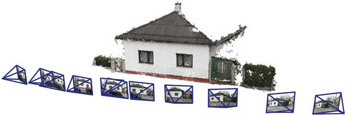
Figure 2.1: A photogrammetric point cloud with location and orientation of the photos. (Source: adapted from [SKMW17])
