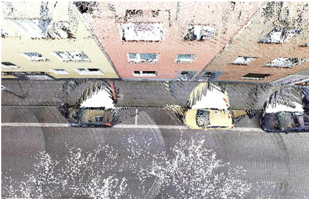
Figure 6.21: The LiDAR point cloud of the street named “Kleiner Griechenmarkt” from above.
