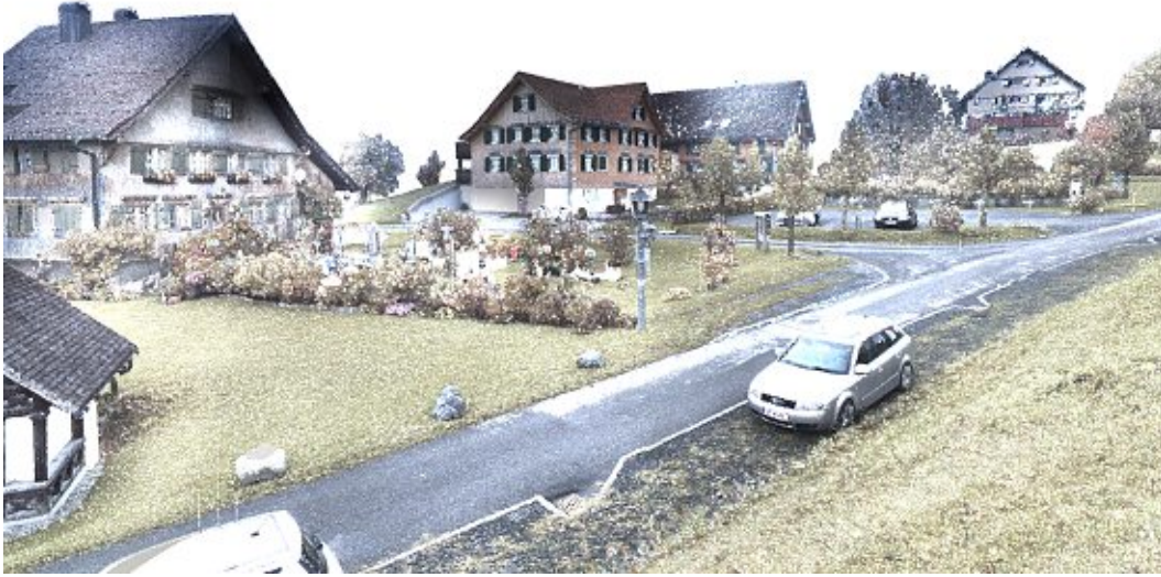
Figure 3.5: A point cloud of the Semantic3d dataset, captured with a laser scanner in a rural area.
