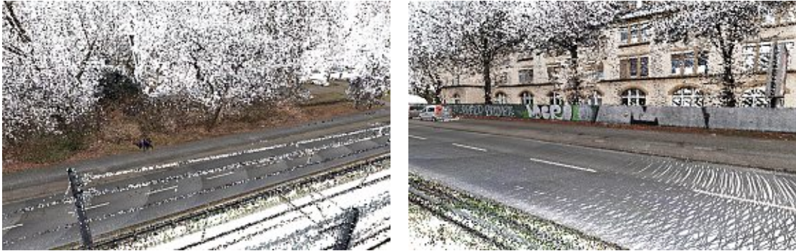
Figure 6.4: The LiDAR point cloud of the two driving lanes of the street in Cologne named “An der Schanz”.
