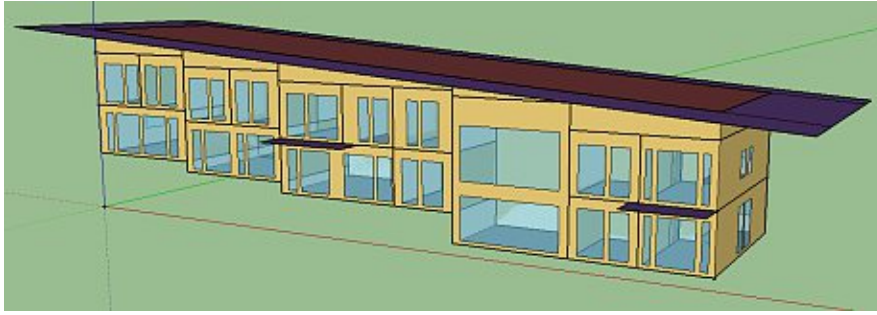
Figure 9: EP+ geometry model for the building compound
