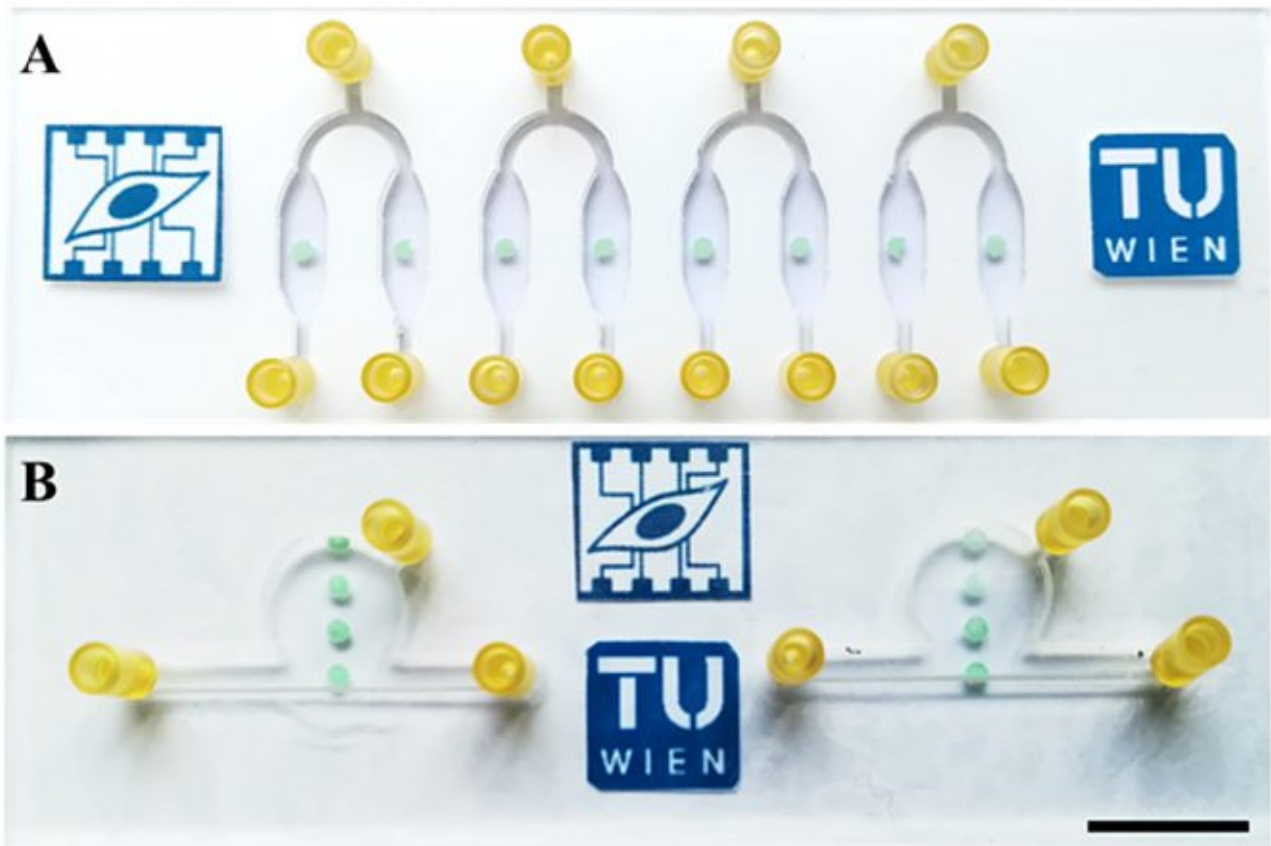
S11: Images of microfluidic devices. (A) Microfluidic glass chip (76x26x2.3 mm) for monolayer culture containing 8 chambers with a sensor spot centralized in each chamber. (B) Microfluidic glass chip (76x26x4.4 mm) for three-dimensional (3D) hydrogel cultures with 4 sensor spots in each chamber. Scale bar represent 10 mm.
