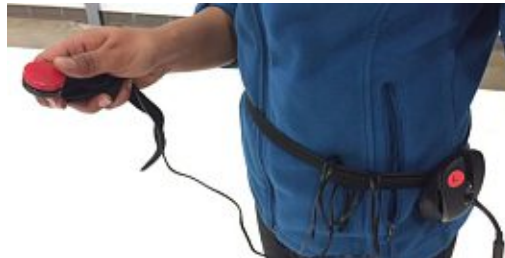
Figure 4. Researcher demonstrating the kick button controller prototype based on a modified Bluetooth wireless mouse.
