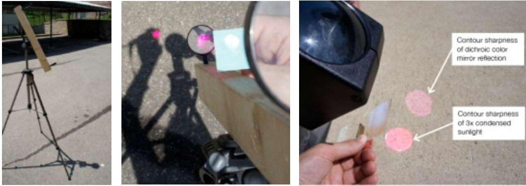
Figure 21: Sunlight projection tests with two double-sided convex lens system and a dichroic color filter (left, middle) and visibility and contour sharpness tests (right), 2014.
