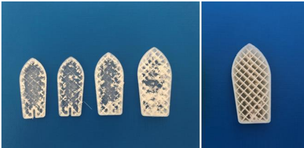
Figure 47. Under extrusion (left) and normal extrusion (right)
