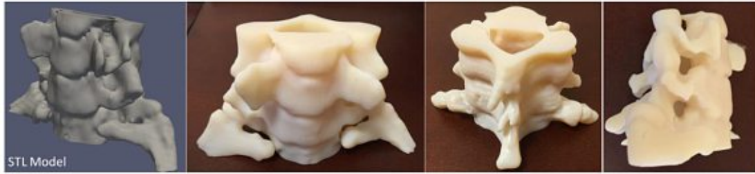
Figure 5. 3D printed MRI-visible cervical spine phantom. From [60]
