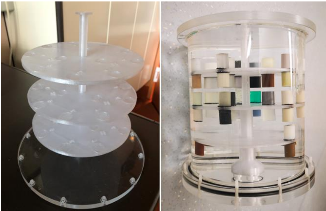
Figure 25. The appearance of the phantom. Left photo: The frame of the phantom. Right photo: The complete phantom (contains 41 cylinders and outer shell, filled with water)
