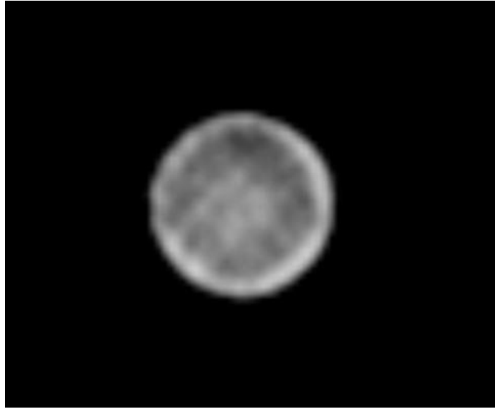
Figure 53. CT image of TPU transparent on Plate C top side position 11 (level: 90, width: 100)
