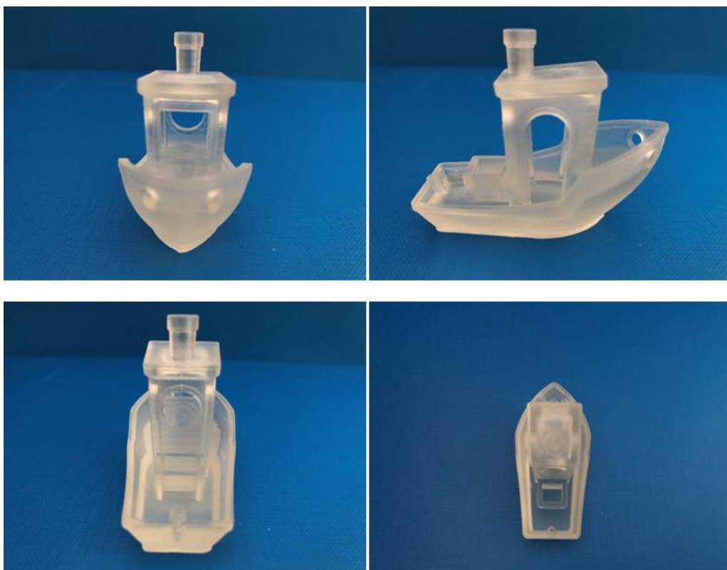
Figure 117. 3DBenchy printed with Wanhao Resin water washable clear
