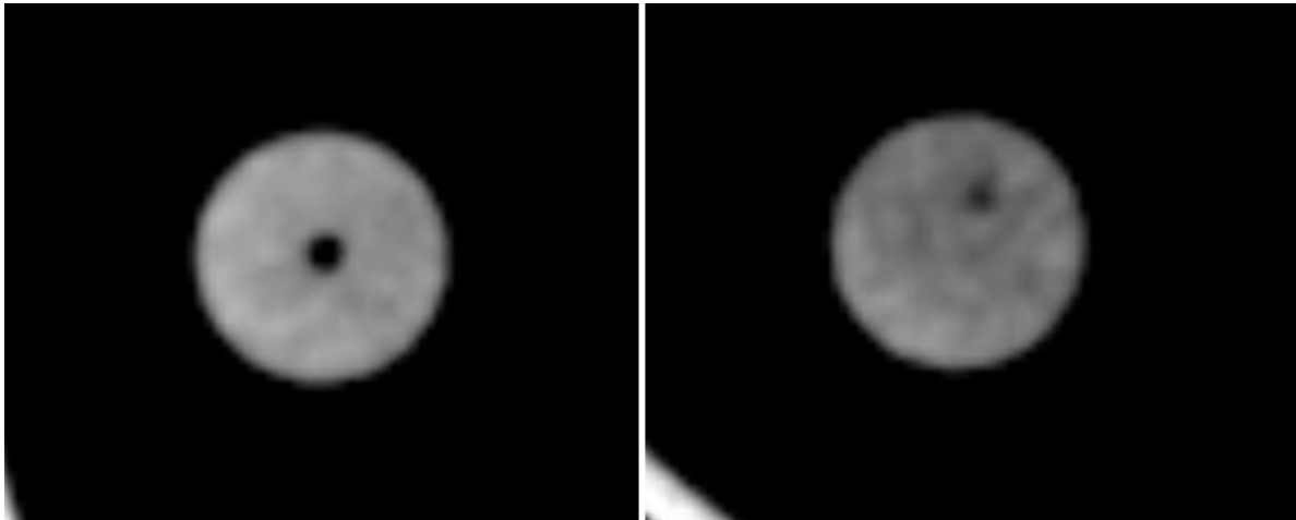
Figure 52. Left: CT image of Anycubic Resin green on Plate B top side position 4 (window settings level: 150, width: 100). Right : CT image of PrimaCreator Resin clear on Plate B top side position 5 (level: 180, width: 100)
