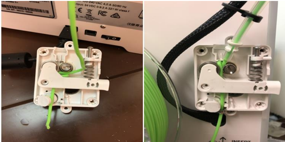
Figure 45. The filament wound around the gear of the feeder twice during the printing of TPU
