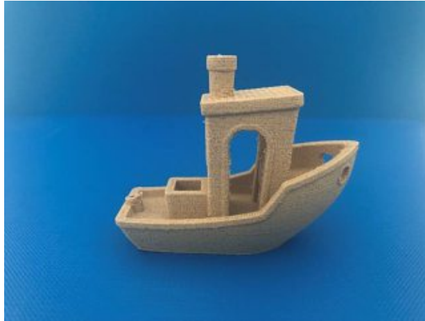
Figure 18. Perfect 3DBenchy (EasyWood material printed with optimal printing parameters)
