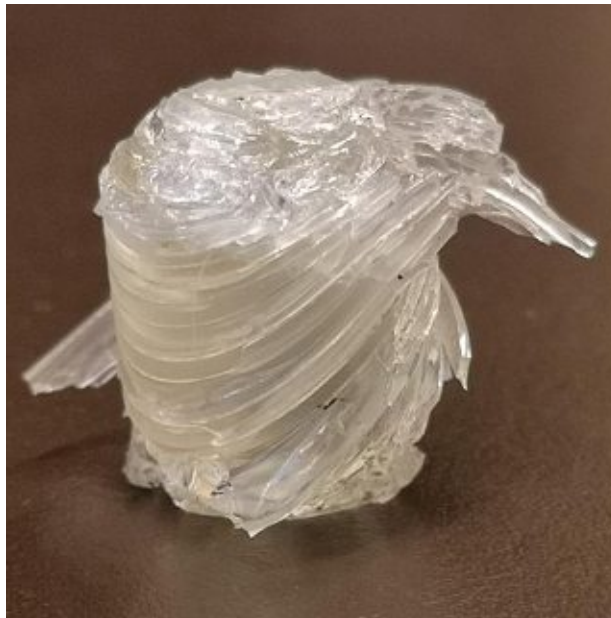
Figure 48. Wanhao Resin printed cylinder after having been immersed into water
