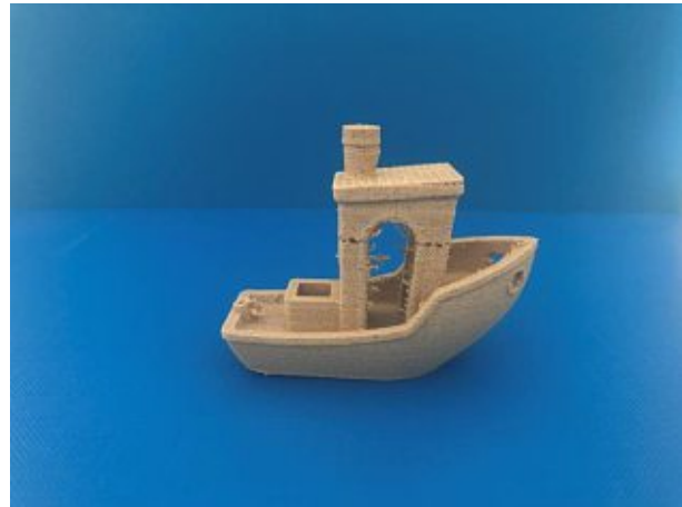
Figure 19. Missing layer and too much stringing (EasyWood material printed with unsuitable printing parameters)
