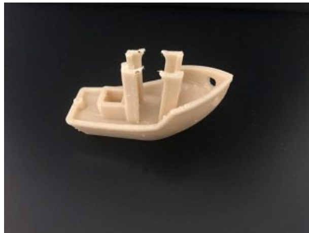
Figure 23. Printing failure (PVC printed with unsuitable printing parameters)
