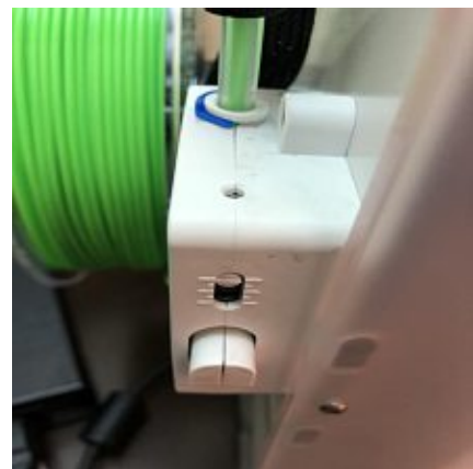
Figure 46. The optimal thrust of the feeder for TPU printing
