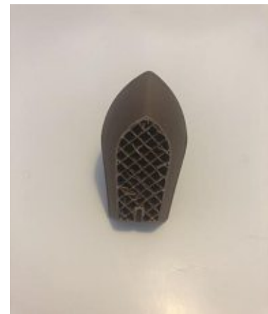
Figure 42. 3Dlac destroyed the bottom of 3DBenchy printed with corkFill material.
