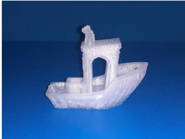
Figure 21. Top deformation (PP printed with unsuitable printing parameters)
