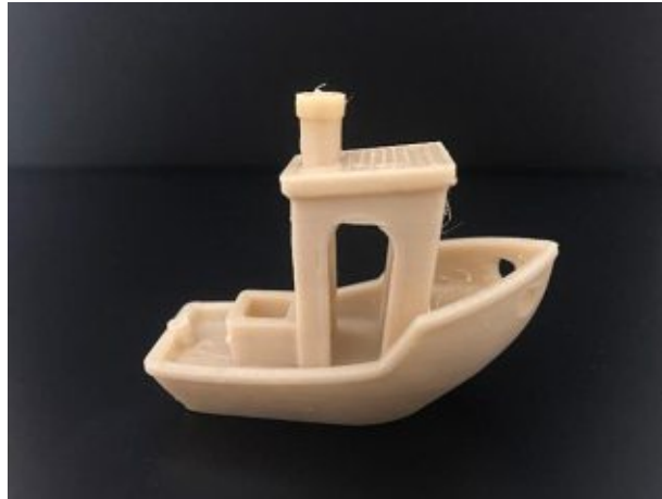
Figure 22. 3DBenchy with good appearance (PVC printed with optimal printing parameters)
