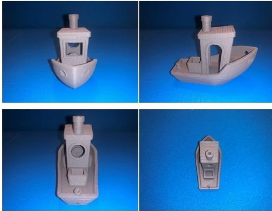
Figure 17. 3DBenchy (printed with steel filled PLA for demonstration)
