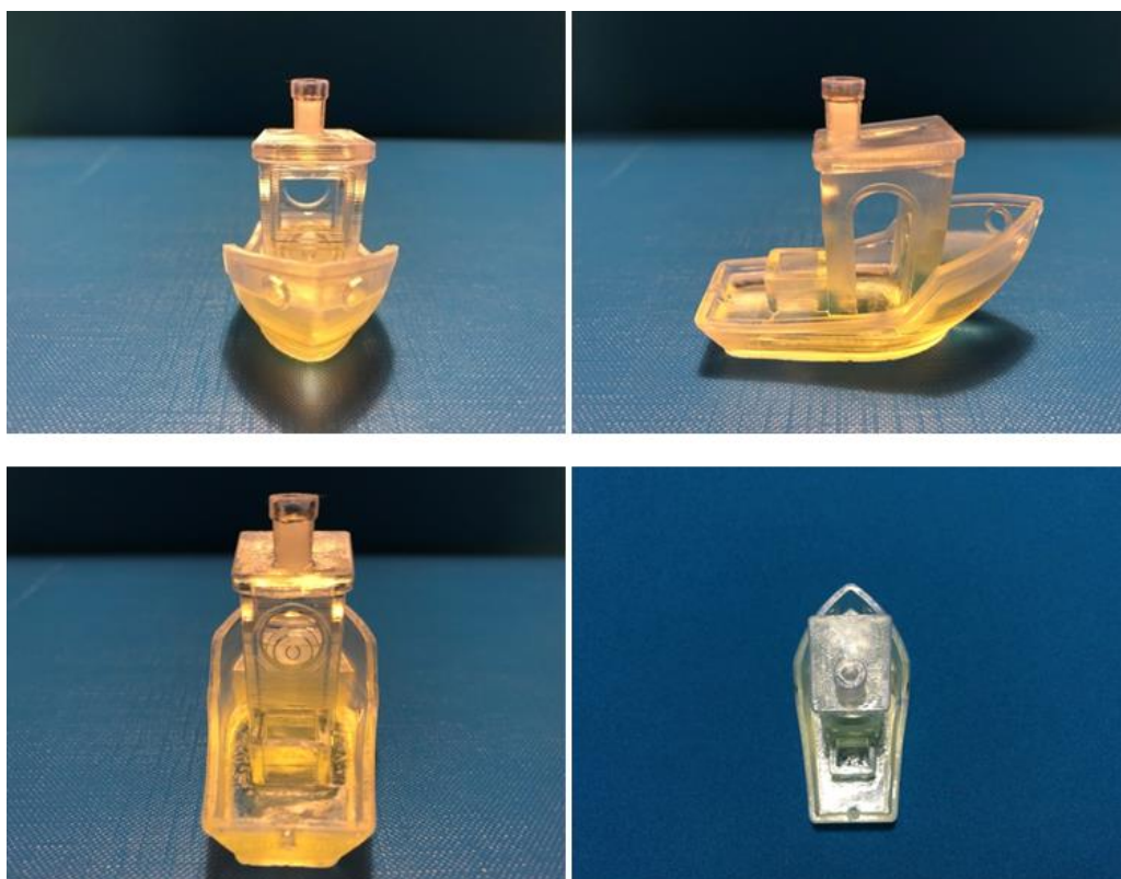
Figure 118. 3DBenchy printed with PhotoCentric3D UV Flexible Resin clear
