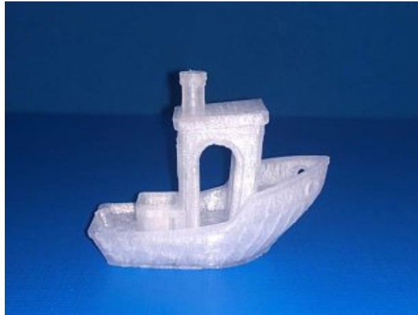
Figure 20. 3DBenchy with good appearance (PP printed with optimal printing parameters)
