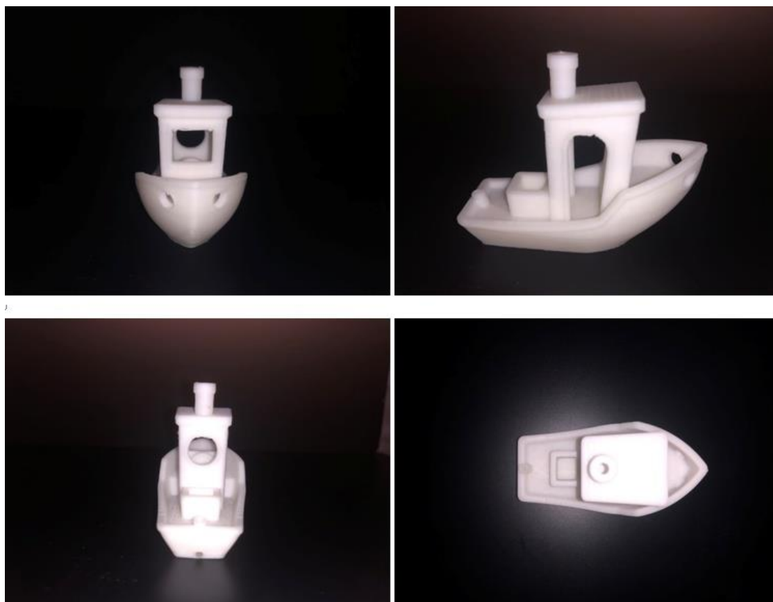
Figure 55. 3DBenchy printed with HIPS
