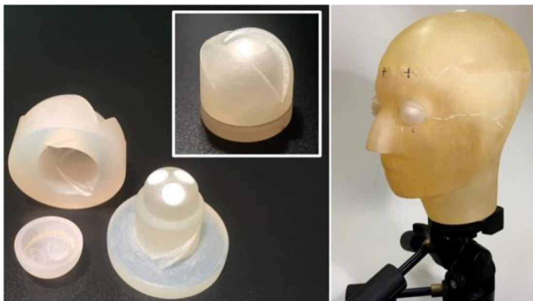
Figure 11. 3D printed anthropomorphic head phantom with eye inserts. From [63]
