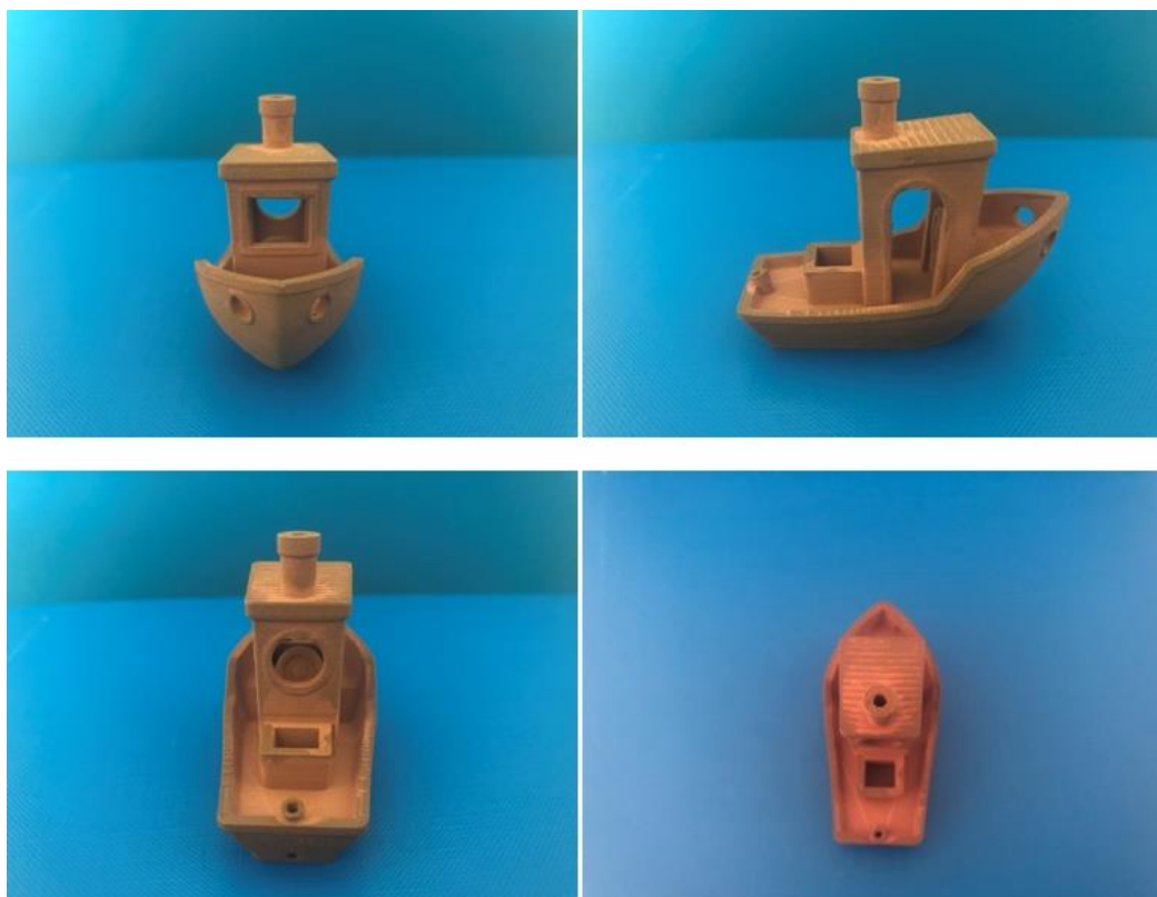
Figure 107. 3DBenchy printed with copperFill PLA (colorFabb)
