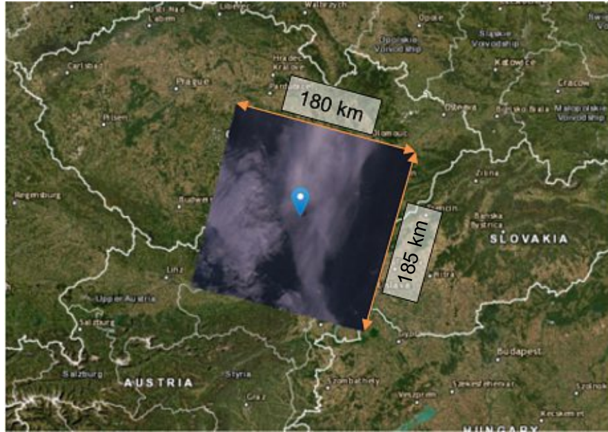
Figure 5: Dimensions of Landsat 8 images at WRS-2 190-026 (Earth Explorer 2020)
