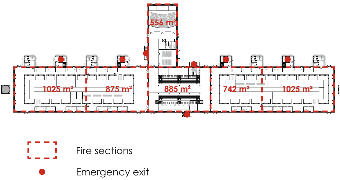
Fig. 99. Fire safety - fire sections and emergency exits
