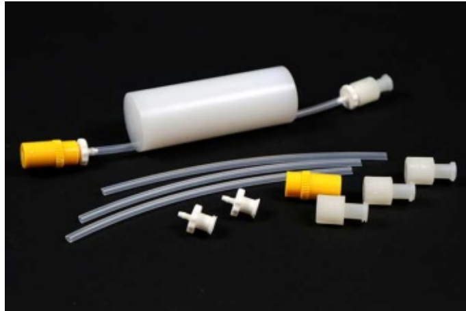
Figure 3.2: Mouse-sized phantom for scatter-measurements based on NEMA-standards. A high density polyethylene cylinder holds the line source, which is created by filling flexible tubing with ^{18}\text{F} FDG. (Source: [37])
