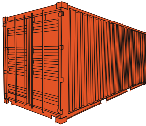
40ft container exterior dimensions: 2.44m wide/ 2.59m height/ 12.19m length
