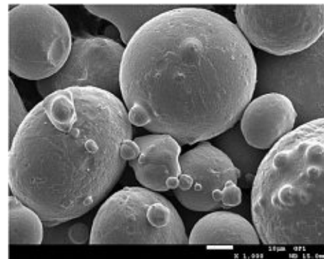
Figure 2 Gas-atomised steel powder (UNS 17400) with typical satellite structure [7]
