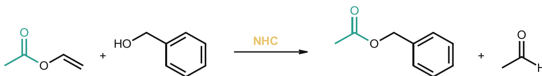
Figure 6. Transesterification using NHC catalysis.
