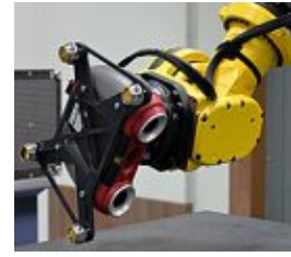
(c) Hybrid system combining active and passive stereo vision
