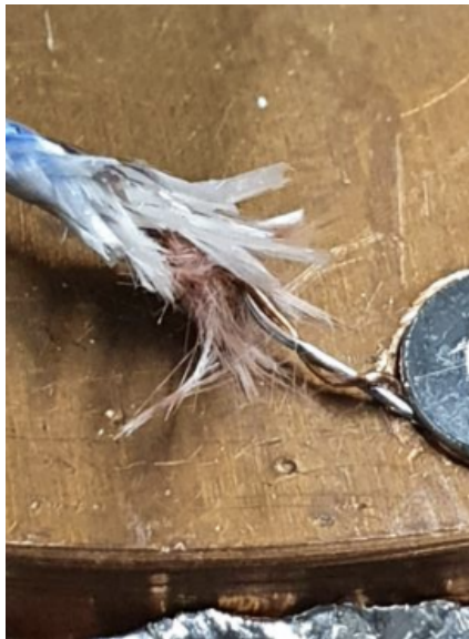
Figure 26: This picture shows how the temperature probe is attached on the copper-plate, to guarantee accurate sensing and mapping of the temperature input.
