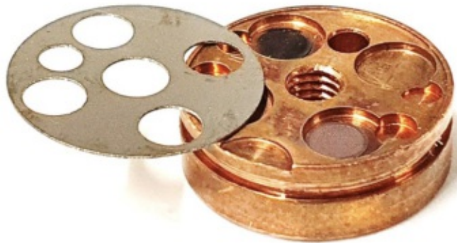
Figure 14: The sampleholder made of oxygen-free copper and magnetic steelplate to hold the sample inside the sampleholder.
