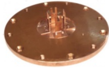
(b) Oxygen-free copper plate and attached oxygen-free copper clips.
