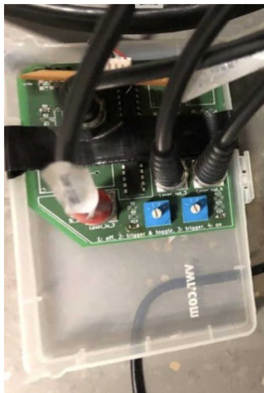
Figure 23: The custom built device to trigger two lasers separately with different possible modes.
