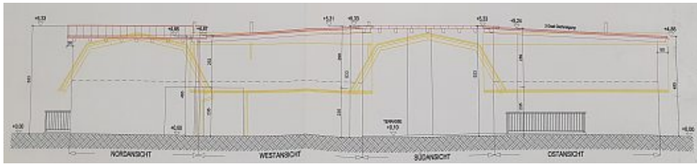
Figure 12: Conversion from mansard roof to a flat roof
