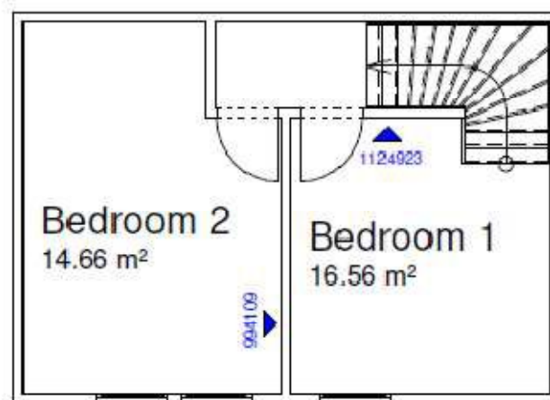
Figure 31: Plan of the first floor of KLG Eschenkogel showing the data logger locations
