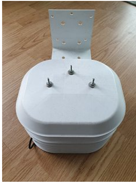
Figure 33: Weather shield for Onset HOBO Data Loggers used to record outside conditions
