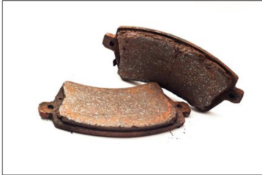
Figure 29: Effect of corrosion on disc brake pads (Hagman, 2021)
