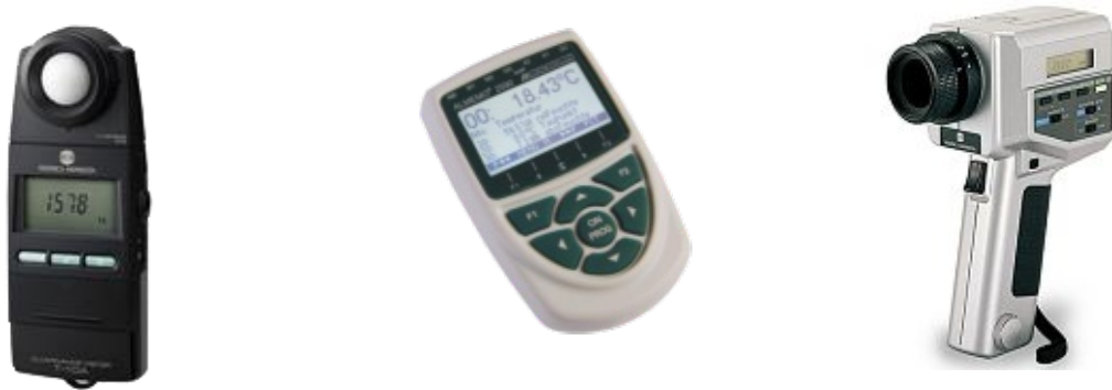
Figure 32: Measurement equipment, from left to right: Konica Minolta T-10A Illuminance Meter, Ahlborn Almemo 2590-4S, Konica Minolta LS 100 Luminance Meter (Konica Minolta Sensing Inc 2013, Ahlborn 2015)
